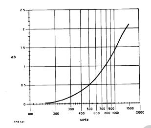
Fig. 5 Insertion loss curve for T connector and probe (typical)
