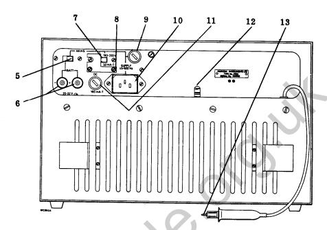
Fig. 2 Controls and connectors on rear panel
