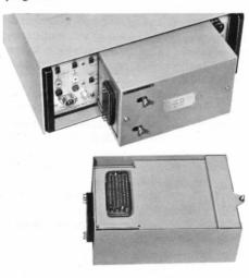
current gain, and true BCD or Decimal code. These modules are the EX 1418 for BCD and the EX 1419 for Decimal code.
