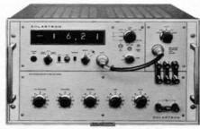
The unit is completely self-contained and measures resistance in the range  $10\Omega-10M\Omega$ .
